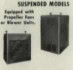
18 sizes and types provide capacities ranging from 50,000 to 450,000 Btu/hr. Features include individual ribbon burners converting heat to separate heat exchangers to provide greater efficiency in less space. Blower equipped units are used to quietly circulate warm air against higher static resistance, permitting the use of ducts.
