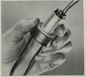
**REMOTE-CONTROL RELAY** operates on 24 volts—cuts costs and copper required to run load lines down to switches. Rated  $\frac{1}{3}$  hp; 15 amp; 125 volts; 5 amp, 277 volts. No need for derating with fluorescent loads.
