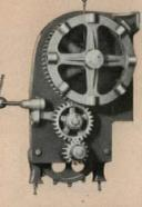
Mahan Release Device for Chain-Gear Operator on Mahan Mechanically Operated Rolling Steel Fire Doors. Fusing of the Fusible Link, which releases the Automatic Closing Mechanism, simultaneously disengages the Chain-Gear Operator.
