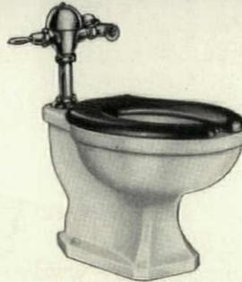
Sanus E-5910-V—Vitreous China, Syphon-Jet Closet, with elongated rim. 1 1/2" top inlet for flush valve, as specified. Projection from wall, 28 1/4". (With round front, projection from wall, 26 1/4".)
