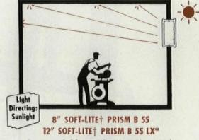
Recommended for sun-elevations where good daylighting and glare control for critical seeing tasks are important.
