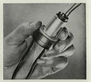
REMOTE-CONTROL RELAY operates on 24 volts—cuts costs and copper required to run load lines down to switches. Rated 1/3 hp; 15 amp; 125 volts; 10 amp, 277 volts. No need for derating with fluorescent loads.
