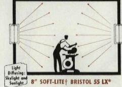
Recommended for all elevations for good light diffusion and transmission and where good thermal insulation is important.
