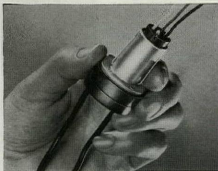
Heart of the 277-volt lighting system is this RR-2 remote-control relay. It will switch up to 10 amperes of fluorescent load. Operates on 24 volts, mounts through 1/2-inch knockout of outlet box or fixture.
