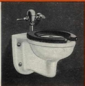
Huburn E-6710-V —Syphon-jet toilet closet with elongated rim. 2" top inlet for flush valve, as specified. Large trapway and 3" outlet. Projection from wall, 25".
