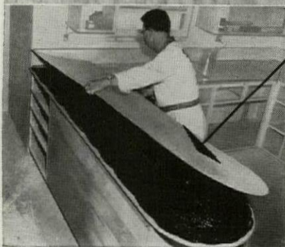
Lamidall is structurally strong—easy to handle, cut and apply. Notice how one man can easily handle a large panel.
