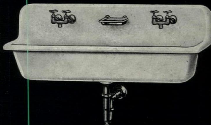
Wash Sink E-1801-A. Enameled Cast Iron. Available with soap dish and single faucet or double faucets, as shown. Lengths: 4', 5', 6'. Width: 18". Height back: 8". Depth inside: 8".
