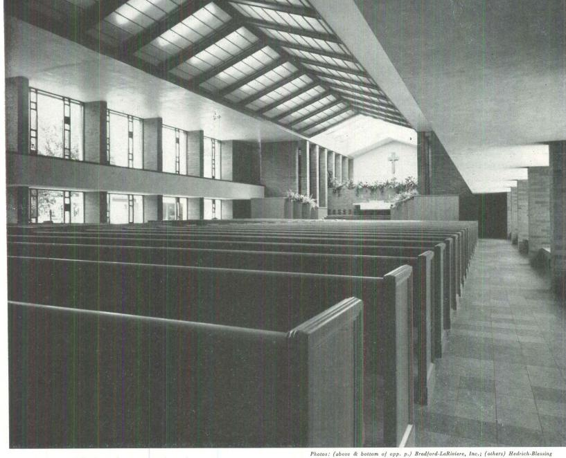
Fluorescent lights behind translucent screen in roof extend skylight effect through church. Brick columns, woodwork and cork floor give warmth to building.
