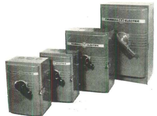
rapidity and force. Grid pins break up the arc, divide it into a series of smaller arcs, dissipating the heat. This type of design results in minimum wear and tear on the contacts. Standard equipment on all models is a felt gasket which keeps out dust and dirt. List prices for the switches range from \$79 for the 2-pole, 240 v. a.c. size to \$133 for the 4-wire, 600 v. a.c. unit. *Manufacturer:* Trumbull Electric, Department of General Electric, Plainville, Conn.
