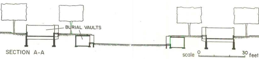
Section through cruciform cemetery shows lower-level mall flanked by retaining walls of vaults and upper-level vaults.
