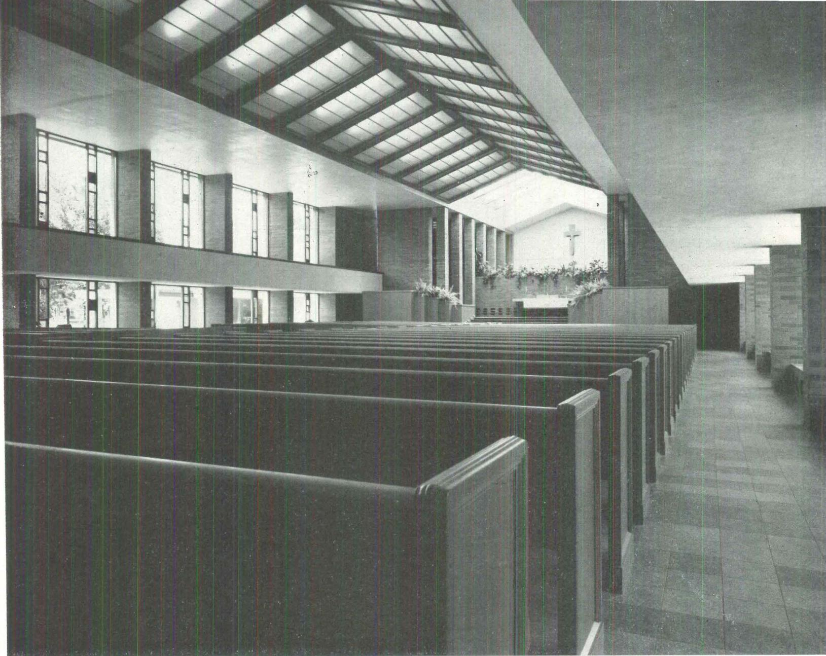
*Fluorescent lights behind translucent screen in roof extend skylight effect through church. Brick columns, woodwork and cork floor give warmth to building.*
