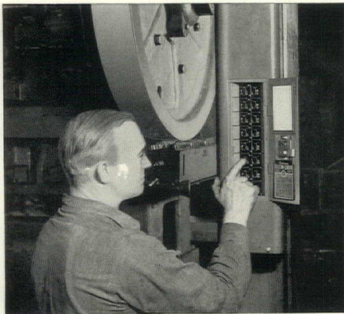
Slim dimensions make it easy to install NPB panels where wall space is limited or not available. They slip easily inside a standard 8" H-beam, fit snugly because of rounded corners. Front overlaps back for deep recessing.
