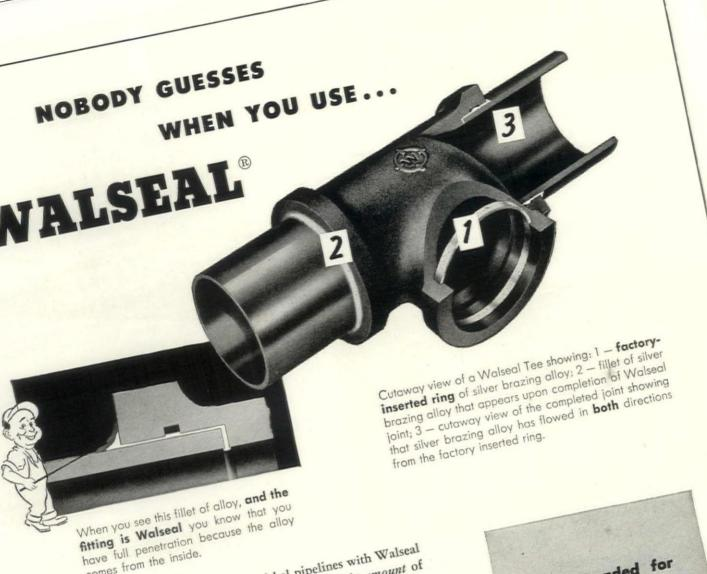
When you join brass, copper, or copper-nickel pipelines with Walseal Valves, Fittings, or Flanges you know you have the right amount of the correct type of silver brazing alloy. The ring of Sil-Fos brazing alloy is factory-inserted in the ports of Walseal products at the time
