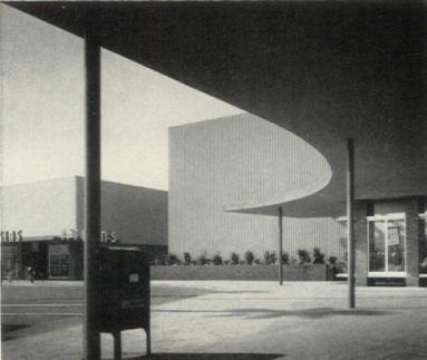
Wedge-shaped tower of department store (left) rises 100' above center, is faced with white porcelain enamel, serves dual function of monument and enclosure for elevator shaft, penthouse, ventilating fans, other mechanical equipment.
