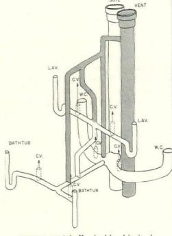
Plumbing stack in Hartford hotel is simpler than Los Angeles Statler, uses 15' less pipe. Major simplification: use of single vent for each pair of fixtures as opposed to conventional venting (designated as "c.v." in diagram below) of each fixture.
