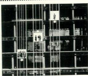
AUTOMATIC BY-PA55—gives Westinghouse Automatic Traffic Pattern elevators even further efficiency. When a down car reaches capacity loading, it by-passes all down corridor calls which are promptly answered by another car.
