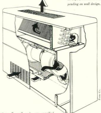
Operation: Fan-coil units are supplied chilled water down to 45° in summer, hot water up to 170° in winter. Fans pull air through filters, blow air up through coil.
