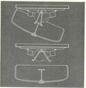
For easy maintenance, fingertip pull on any side drops bowl to safe position, held by the Tortiontite\* spring. Can be removed entirely by compressing spring.
