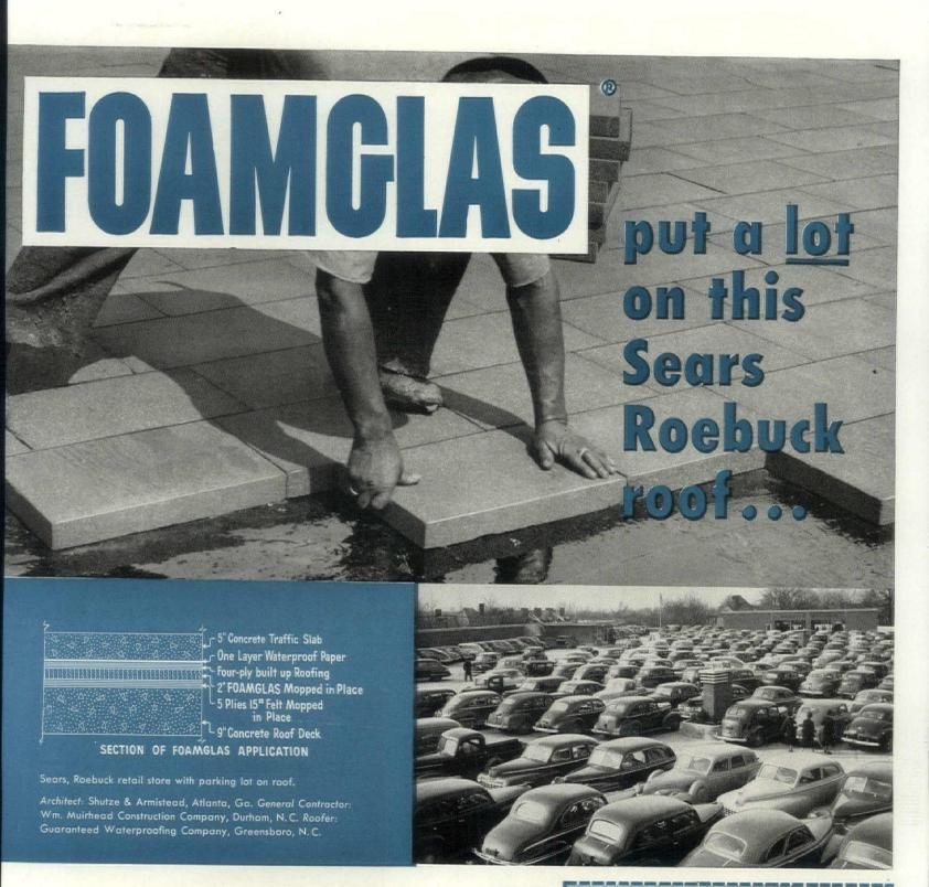
By putting the parking lot on the roof Sears, Roebuck and Co. cut land needed in half, but it took FOAMGLAS insulation to make it practical for their new Winston-Salem store. Other insulations lack compressive strength enough to withstand such a load, while each 2" x 12" x 18" block of FOAMGLAS used theoretically could support the weight of nine Sears' customers' cars.
