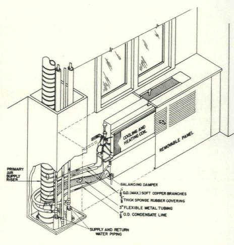
No motor, fan or filter is nececessary; high-velocity conduit-supplied air induces secondary room air into unit. Baffled plenum inside unit is for suppressing air noise. Supply water temperatures in coil range from 50° in summer to 170° in winter.
