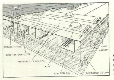
Every cell in the structural subfloor is a potential wire raceway. Electrical equipment involved in any interior arrangement, or rearrangement, is easily accommodated.
