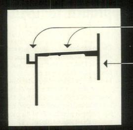
Made of Extruded Aluminum with welded joints for clean lines, enduring beauty and great strength.
