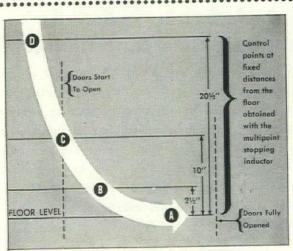
**SYNCHRO-GLIDE LANDING CONTROL** — brings cars to a bird-like stop . . . fast, smooth, accurate. Power-operated doors are synchronized to open as the car is landing.
