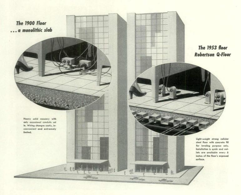
Q-Floor provides truly modern structural floor construction because it permits quick change of electrical outlets at 6-inch intervals over the entire building. This effectively eases the time and expense of moving equipment and partitions. The advantages of Q-Floor on the construction job are many, and
