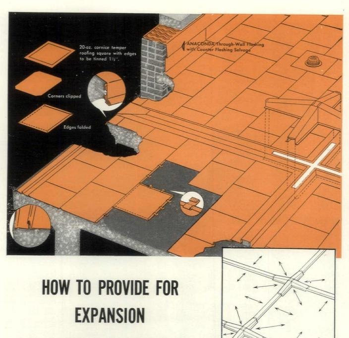
in watertight, flat seam copper roofing
