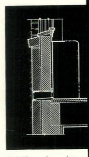
Air intake can be anywhere behind unit. Units average 12" in depth, can be recessed depending on wall design.
