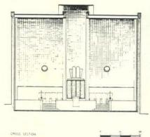
Sections and plan show how rising curve of temple roof from behind ark is supported on large tapering steel beams, and how temple, foyer and assembly can be combined by shifting movable partitions. School area for 400 pupils has been built, but library and nursery which jut out into interior garden have not yet been added.
