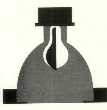
no other recessed lighting instrument offers all the practical advantages of Century's series 930 ellipsoidal Downlite ... compact, low in cost, uses general service lamps... bulb just screws in from below-no plate to open ... eve comfort is assured by the extremely low brightness of the opening-which is small . . . the bottom of the unit is absolutely flat and smooth (no bumps in the ceiling plane) and the precision reflector is Alzak Processed for permanent efficiency
