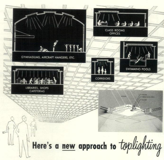
Skytrol glass blocks—a new toplighting medium—now give the architect a sturdy, flexible design unit that overcomes these three big objections to skylights: high heat loss, condensation and costly maintenance. The double cavity created by the fibrous glass insert gives the Skytrol Block a "U" value of .44, thus reducing heat loss and practically eliminating condensation. These new skylight blocks are self-cleaning, and they reduce other maintenance costs to an absolute minimum.
