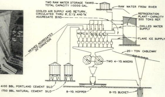
Inside the ice plant at Folsom dam: Ice forms on revolving steel cylinder, is flaked off (1), fed to bucket elevator by screw conveyor (2), thence to storage bin at top of batching tower (3) from which it drops along with other ingredients into mixers (4) and is finally conveyed to the dam in 8 cu. yd. bucket hung from 20 ton cableway (5).
