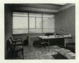
Small offices can be created by partitioning anywhere within the 3'-93/4" window module along continuous window walls.
