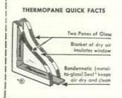
Thermopane insulating glass is widely and successfully used. Thermopane with ½" of dry air hermetically sealed between two panes has twice the insulating value of single glass. This minimizes chilliness, drafts and heat loss at windows in winter. Thermopane cuts airconditioning costs by reducing the amount of heat entering during summer. It cuts out 44% more noise than single glass. Write for Thermopane literature. Libbey-OwensFord Glass Company, 4293 Nicholas Building, Toledo 3, Ohio.
