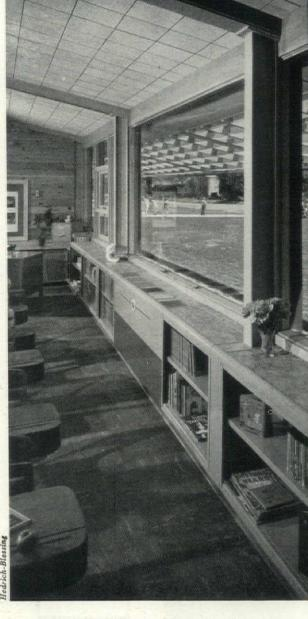
Heating and ventilation is integrated with architecture in Columbia, Wis. classroom by Architects Weiler & Strange. Generous sunshade minimizes periodic solar gain. Glass is largely fixed. Unit ventilator beneath window supplies mixture of outdoor and recirculated air, controlled to heat or cool room as necessary. Location of continuous ventilator return behind flanking cabinets traps any downdraft from windows before it can enter room.
