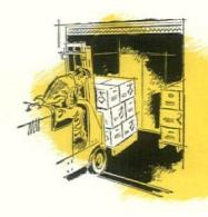
1915—The first self leveling, or Micro-Drive, elevators were developed by Otis engineers and enable passenger and freight elevators to be brought to an accurate stop at floor landings and to maintain this level automatically. This development saves time, eliminates the stumbling hazard and permits trucks to run smoothly on and off an elevator platform.
