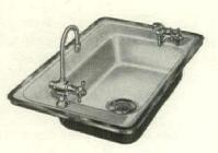
• The HAWS Receptor is cast iron—beautifully finished in acid resisting white enamel. Stainless steel mounting rim prevents water running onto table or cabinet top and affords a water tight bond between sink and top surface.
