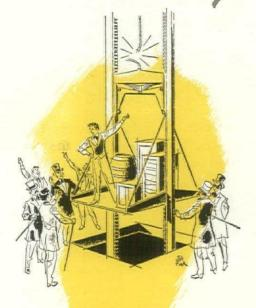
1853—Elisha Graves Otis invented the first safe elevator. It was equipped with a safety device to prevent the elevator from falling if the ropes should break, which was a frequent occurrence in those days. Until a safe elevator became available, buildings and cities had grown vertically only as high as people were willing to climb stairs.
