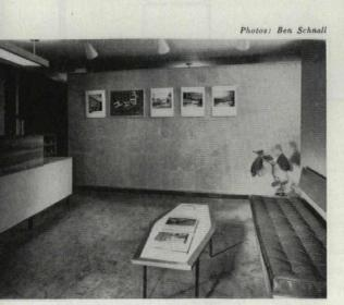
Reception room partition is perforated cement asbestos board acoustically treated.
