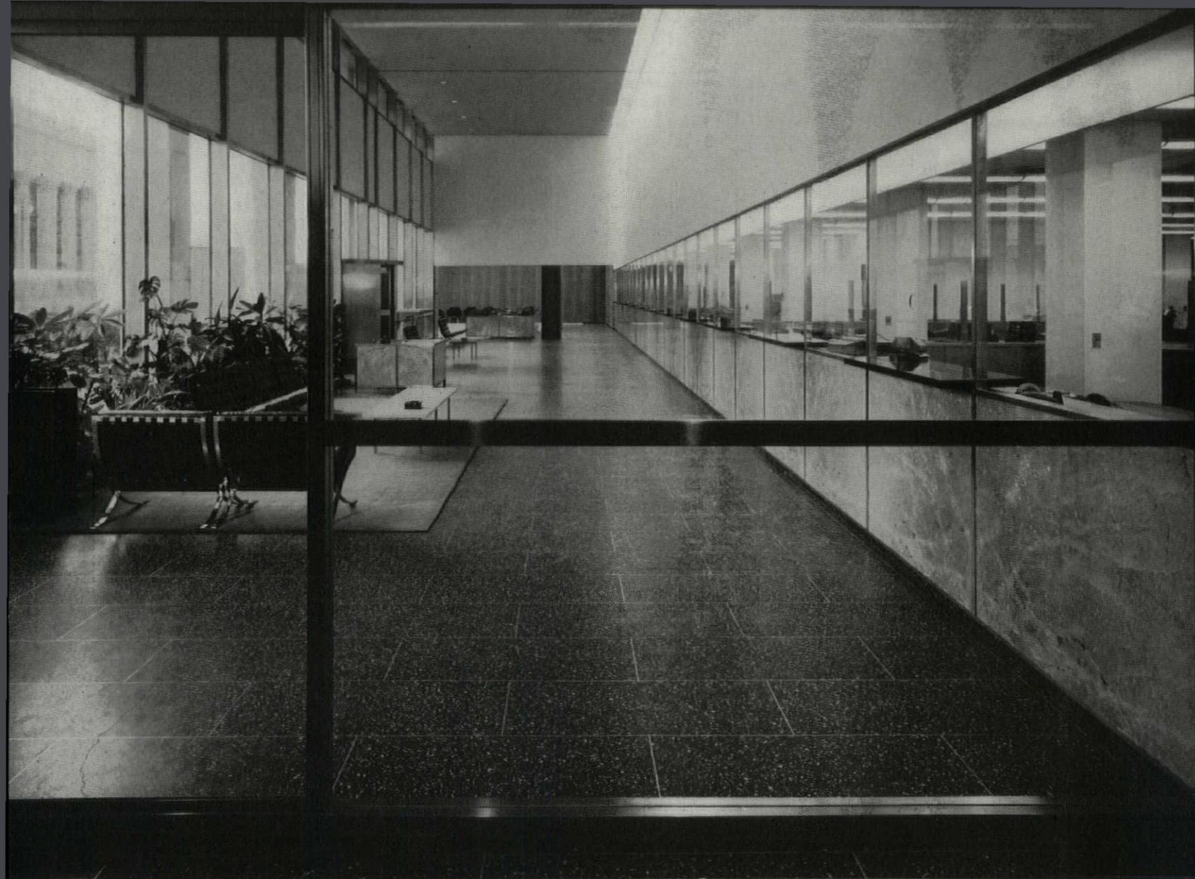
In well-lighted lobby, note second high row of small windows above solid panels in wall at left. All-glass front would have produced glare and spoiled the space effect of the room.
