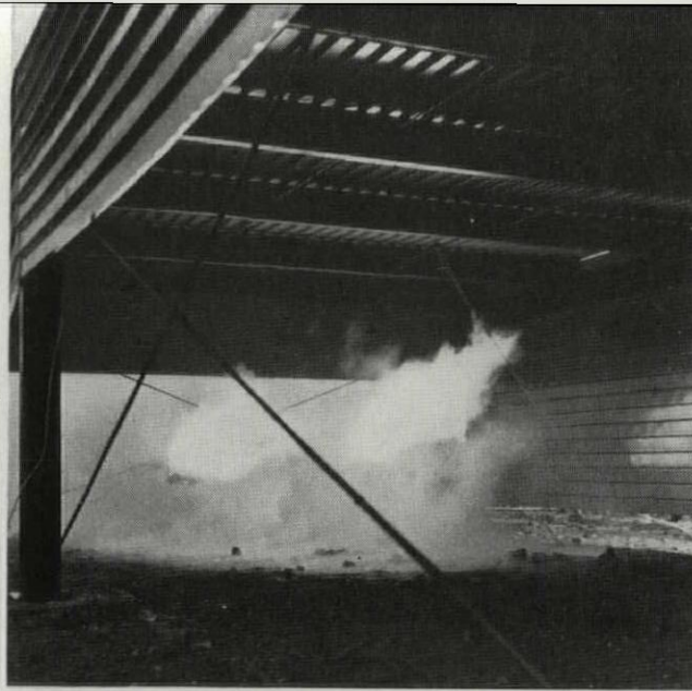
Typical test bays with oil burners at end just ignited. Framing and sprinkler layout shown on left, where lettered squares indicate cut-out samples removed for examination after each test. Eight thermocouples are strategically placed to supply temperature-time readings throughout tests.
