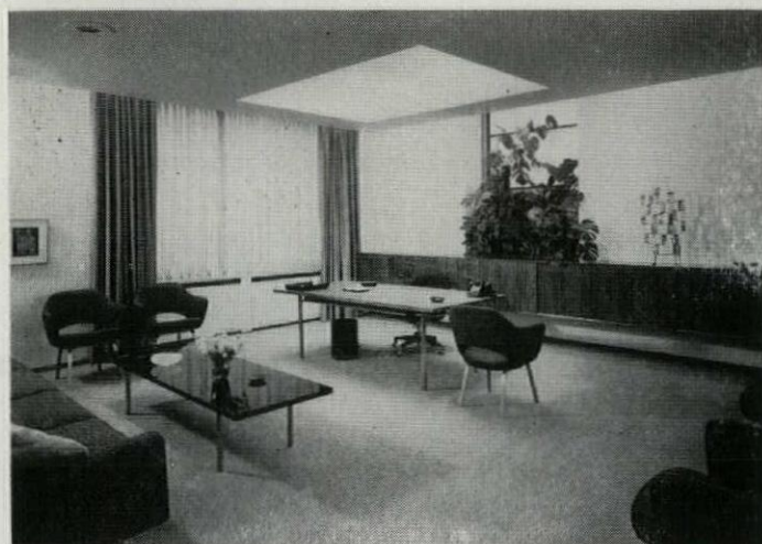
Vice president's office has window at left looking out on garden, and hung acoustic plaster ceiling bounded by a lighting cove which washes the walls with light. A rectangular louvered panel of recessed lighting gives 100 foot-candles to the desk.
