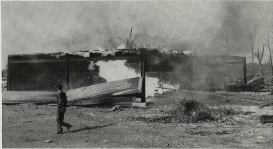
End of Test I, burning vapor seal dripped through roof, side panels collapsed
