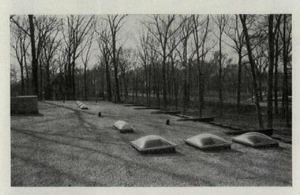
**WASCOLITE SKYDOMES** are lightweight, prefabricated units that do <u>not</u> require special roof construction. Their extruded aluminum frames have a built-in weepage arrangement that assures leakproof installation. Skydomes are weatherproof, shatter-resistant and virtually self-cleaning. They can be installed in minutes — using only a screwdriver.
