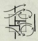
Cold winter winds in southeast and south central US (opposite direction from warm winds) are blocked by same wall that directs summer breezes into rooms. Diagrams show wind diversion in plan and section; photo (above) shows smoke test with model at Texas Engineering Experiment Station. Locales where summer and winter winds come from same direction (as at Columbus) require adjustable louvered windbreak. Northern areas, such as Duluth, require only windbreaks for winter weather.
