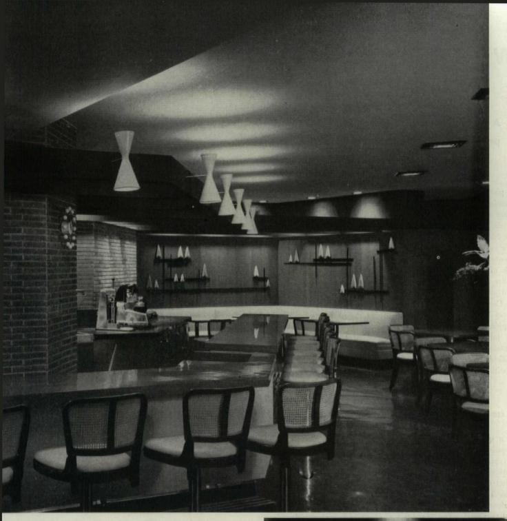
Columnlike stack of brick standing in center of fountain space hides entrance to kitchen on way in, is also fulcrum for entire design. Two ceilings, one white-troweled plaster, one yellow-gold acoustical plaster, intersect on its line. Counter and open redwood beams radiate from it. Cost of restaurant; \$48,136, or \$20 per sq. ft. Contractor: De Martini Bros.
