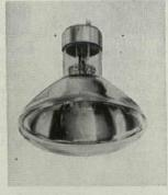
toast sandwiches. Equipped with two separate filaments, the 1,550-w. unit can be operated at three different wattage - 650, 900, and 1,550-permitting close control of the infrared output. Made of thermal and shock-resistant Vycor glass, the lamp is not affected by spattering liquids during operation. Its built-in continued on p. 244
