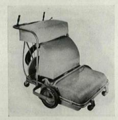
ten seconds and the big dust-collecting bag requires infrequent emptying. Powered by a 2 hp gasoline engine the *Turbo-Sweep* is self-propelled and has a silencer. Its 40" sweeping width permits cleaning of 40,000 sq. ft. of floor area an hour. Price, F.O.B., Springfield, Ohio, is \$648; a riding "sulky" (optional) costs \$45. *Manufacturer:* Parker Sweeper Co., Springfield, Ohio.
