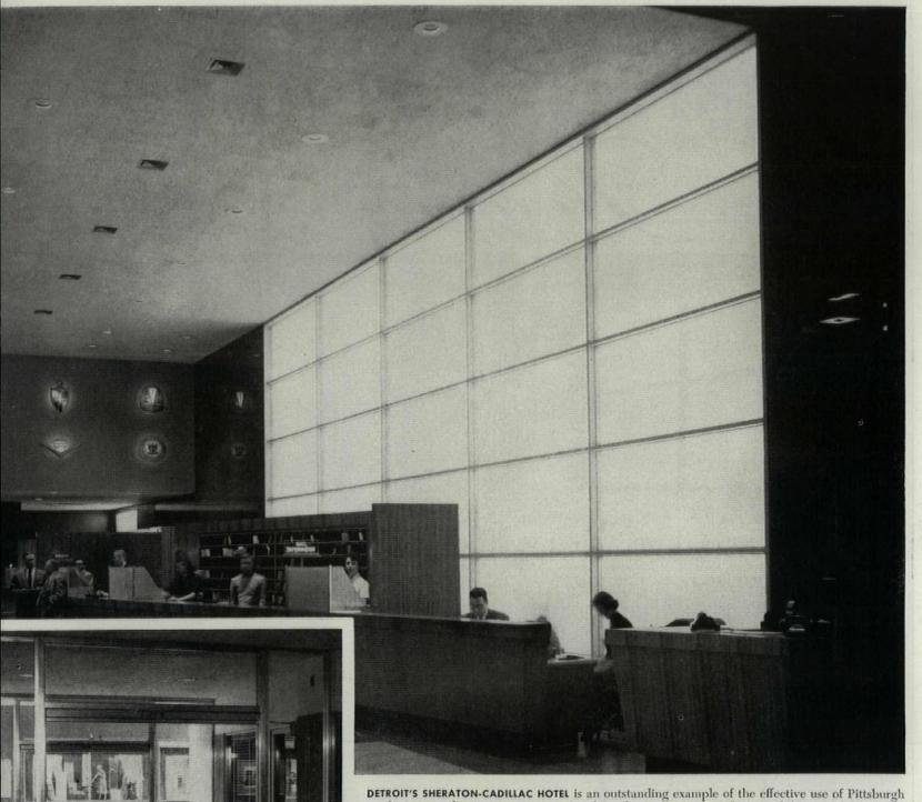
products in modernization programs involving large structures. A feature of this remodeling is the lobby which includes forest green Carrara Structural Glass, Pittco Store Front Metal construction and a translucent "glass wall" glazed with Mississippi Softone Bondlite. This results in an interior that is tremendously appealing and distinctive. Architect: Mary Morrison Kennedy, Boston, Mass.
