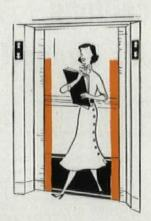
Only AUTOTRONIC elevators have car and hoistway doors with an *electronic zone of detection*. It is a proximity zone that extends in front of the leading edges of both the car and hoistway doors up to shoulder height. Naturally, it is invisible to the passengers. (See phantom drawing at the left.)
