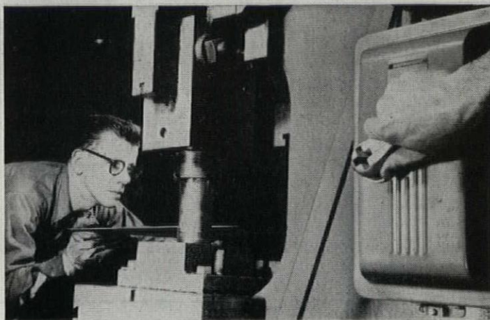
AB-1 Circuit Breaker —protects circuits and students wherever power equipment is used. No fuses to replace. No danger of over or under fusing. After overloads, service is safely restored by flipping handle on outside of enclosure.
