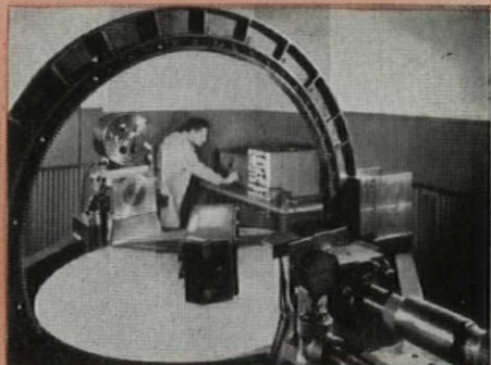
Roll Test Model for Developing Airplane and Rocket Flight Control Devices
