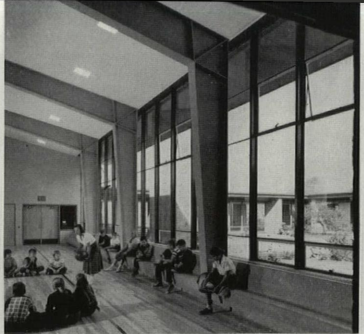
Playroom is framed with rigid steel bents painted bright coral. Tempered glass windows absorb knocks, have proved safe. Emphasis is on sports participation so resting benches are only seating.
