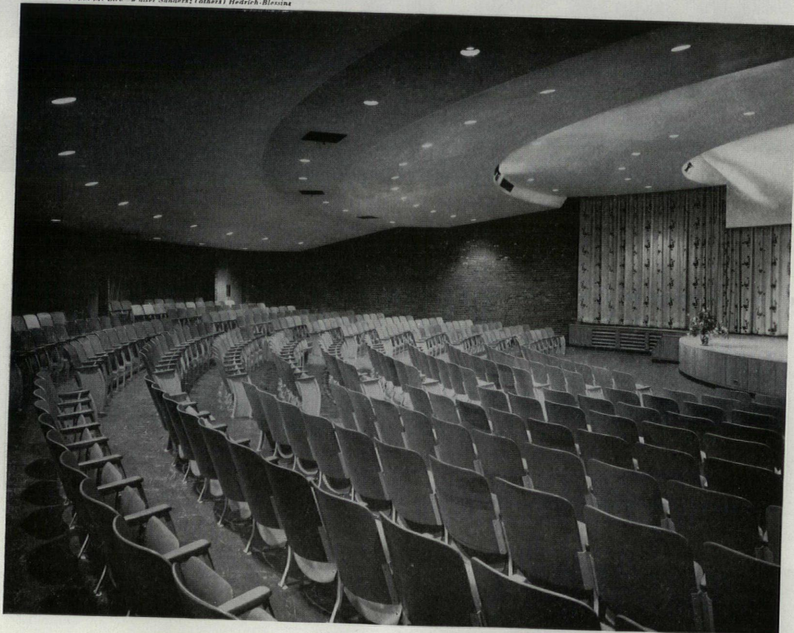
Auditorium stage can have three scenes set up simultaneously, one in large center portion, one in 9' opening to each side. Ceiling is finished in acoustic and hard plaster. Capacity: 420.
