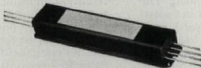
LAMP BALLASTS —This one shown above (rated 265 volts) for use with two 40-watt rapid-start lamps, designed for use with 277-volt systems.
