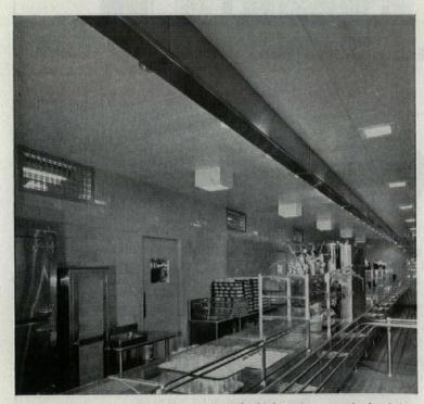
The high sanitary standards of the cafeteria's serving area are fully met by the easy-to-clean Arrestone ceiling. Installed by mechanical suspension, sections of this ceiling can be removed for repairs on concealed piping or wiring.
