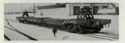
Special railroad car has low platform and pedestal at either end to support trailers. Photo (at right) shows piggy-back train on New Haven's regular New York-Boston run pulling out of terminal on outskirts of New York. Train beats highway time for the run, and shippers save money due to less handling.
