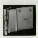
WIDE-THROW HINGE. Offsetting a 1-3/4" door at a 90° angle, Stanley's BB 266 hinge allows full clearance of hospital corridor and bedroom doors for easy passage of beds and carts, Its wide-throw eliminates tacking of protective metal strips on doors. The self-lubricating ball-bearing hinge is made of heavy wrought steel in all standard finishes. The Stanley Works, New Britain, Conn. (Sept. '53, p. 236).
