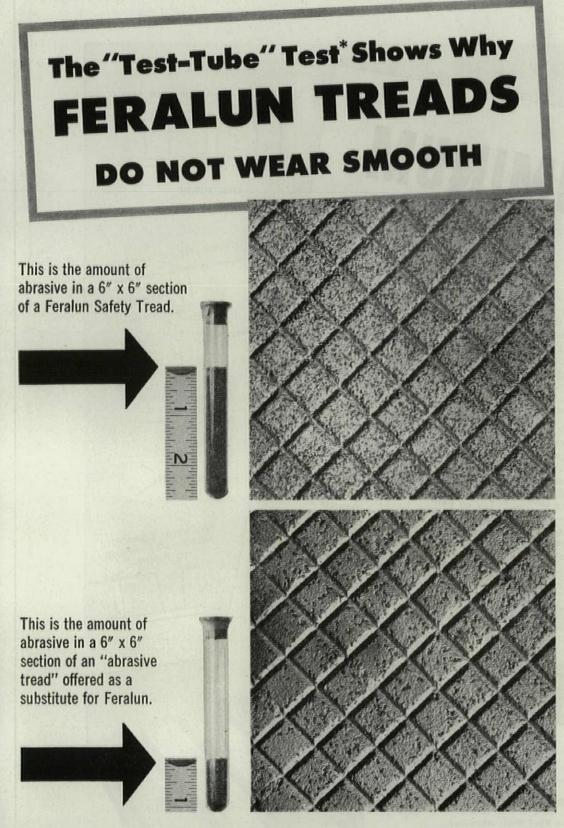
The life and non-slip effectiveness of an abrasive tread depend on the amount of abrasive it contains and on the even distribution of the abrasive over the wearing surface. To many, the two treads above may look alike, but when the abrasive is removed and compared the difference between them becomes apparent.
