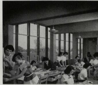
**Classrooms** have full windows on north, as in homemaking room (above). Biology laboratory (left) shows typical south wall of classroom, with 7'-6"-high, partition at corridor, 3'-6"-high opening above. Classroom color schemes vary; most have three wall and tackboard colors and light-colored asphalt tile flooring. Some floors have inlaid color strips to aid in lining up movable furniture.
