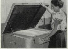
A positive photographic intermediate is produced directly by exposing the "paste-up" in contact with Kodagraph Autopositive Paper, then processing the print in standard photographic solutions. No negative step . . . easy room light operation.
