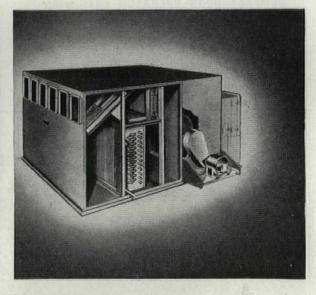
Trane Multi-Zone Climate Changers are air handling units which can heat, cool, humidify, dehumidify, ventilate and filter air (singly or in combination) for as many as six different zones at once. 28 models, 450 to 23 400 cfm. to 23,400 cfm.
