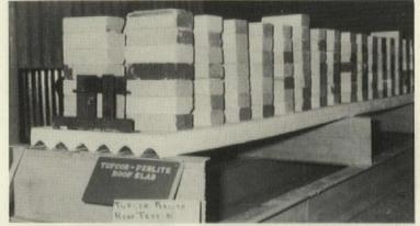
6. LOAD TESTS show the tremendous strength of a roof slab similar to that used in the fire test. After ½ million cycles of repeated loading, from zero to full design live load, the slab was loaded until it finally failed at 273 psf of 8.9 x design live load! Based on 30 psf live load, the ultimate factor of safety of the Tufcor roof slab is 9.0. (See Pittsburgh Testing Laboratory Test No. 282-T-403.)
