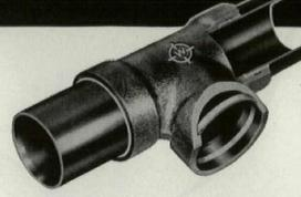
Cutaway view of a Walseal Tee showing: factory-inserted ring of silver brazing alloy; fillet of silver brazing alloy that appears upon completion of Walseal joint; cutaway view of the completed joint showing that silver brazing alloy has flowed in both directions from the factory-inserted ring.
