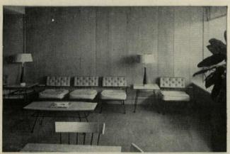
EASY-TO-INSTALL OAK PLANKWELD adds a cheery background to this unusually pleasant waiting room. Plankweld can be installed on any wall with special metal clips which hide nails.
