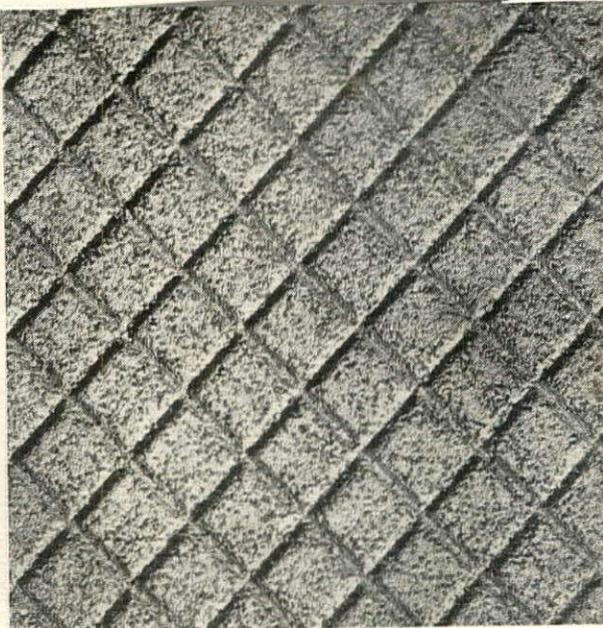
This is the amount of abrasive in a 6" x 6" section of an "abrasive tread" offered as a substitute for Feralun.
