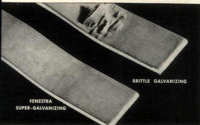
**BEND TEST** demonstrates the durability of Super Hot-Dip Galvanizing. It won't crack. With some types of galvanizing, when the steel is bent, then straightened, the galvanizing cracks open, leaving the steel vulnerable.
