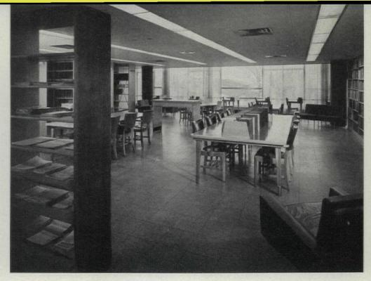
special reading rooms on north side have same economical 7'-8" ceiling height as stacks and offices on the south, afford spatial contrast with 19' general reading rooms (photo below). Light levels are maintained at a high 60 foot-candles in special reading rooms, 45 foot-candles in two-story reading areas,
