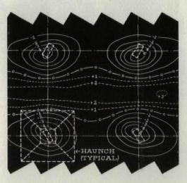
Photoreflective analysis shows reinforcing steel intensity required under loading.
