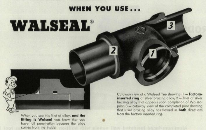
When you join brass, copper, or copper-nickel pipelines with Walseal Valves, Fittings, or Flanges you know you have the *right amount* of the *correct type* of silver brazing alloy. The ring of Sil-Fos brazing alloy is *factory-inserted* in the ports of Walseal products at the time of manufacture.
