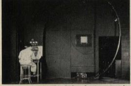
Because of its light-selecting principles this new block has a much lower surface brightness than other glass block. Maximum surface brightness as measured at the Daylighting Laboratory is less than 1400 foot-lamberts.
