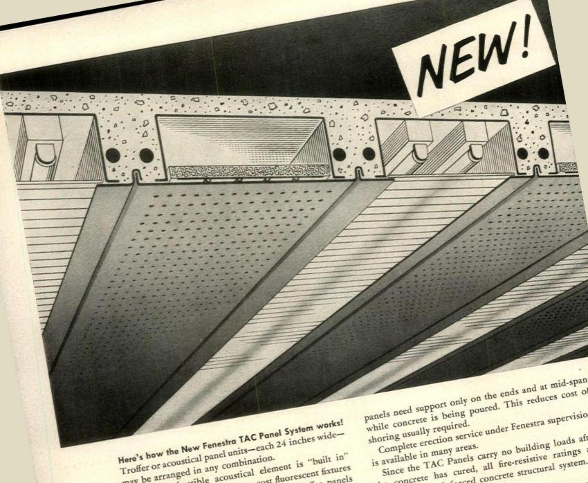
A noncombustible acoustical element is "built in" may be arranged in any combination. the acoustical panels. Minimum-cost fluorescent fixtures and plastic diffusers are installed in the troffer panels
