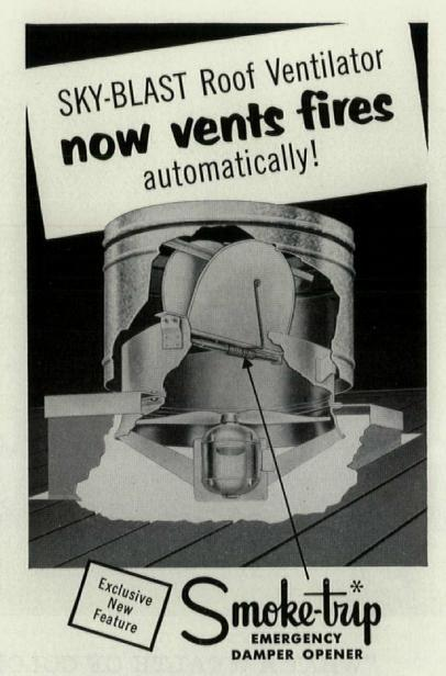
This powerful roof ventilator is now available with an important new safety device... the Smoke-Trip emergency damper opener developed as the result of recent fire studies. Heat from an uncontrolled blaze inside the building will melt a fusible link, releasing high-torsion springs which open the dampers. Treacherous smoke, heat and fumes which hinder fire fighters are vented to the outside air.
