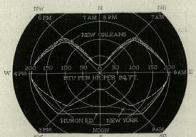
Compass rose shows maximum solar heat in Btu per sq. ft. per hour, falling on walls facing in all directions at latitudes of New Orleans, New York, and Huron, S.D., on Aug. 1. Heat is lowest on walls facing due north and due south.
