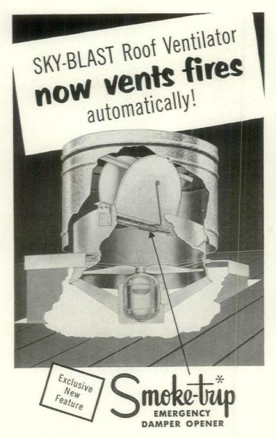
This powerful roof ventilator is now available with an important new safety device . . . the Smoke-Trip emergency damper opener developed as the result of recent fire studies. Heat from an uncontrolled blaze inside the building will melt a fusible link, releasing high-torsion springs which open the dampers. Treacherous smoke, heat and fumes which hinder fire fighters are vented to the outside air.
