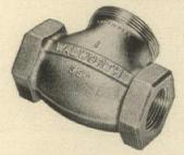
EXTRA STRONG BODY: Made of Composition M (ASTM B61) bronze. Thick walls and rugged hexes provide a high safety factor. Valves undergo hydrostatic shell test of 1,200 psi.
