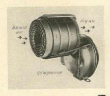
dryer consists of a 1/6th hp hermetically sealed unit. It weighs 45 lb. and operates on 110 A.C. current. As air is pulled over the refrigerated coils of its compressor, moisture condenses and is caught in a receptacle or carried off through a tube. At 90° F., 90% humidity, the air dryer removes 3 gal. of water every 24 hours, yet consumes about as much electricity as a 200-w. bulb.
