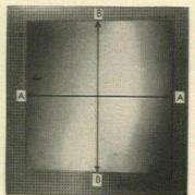
PROFILE MEASUREMENTS of stainless steel wall panels reveal flatness required to eliminate unsightly waviness
