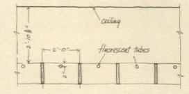
SELECTED CEILING has vertical baffles and exposed fluorescent tubes which will operate at half power to minimize glare.
