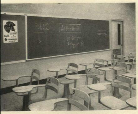
INSTALLED COST of Weldwood Chalkboard is usually less than for ordinary chalkboard; it needs no costly fixed grounds or other surface preparation: it mounts directly to wall.
