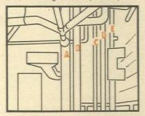
A. 8" soil stack. B. 6" vent. C. 3" hot water. D. 4" cold water. E. 3" waste for future use. Laterals to soil stack are 4". All sanitary drainage lines are Type M.
