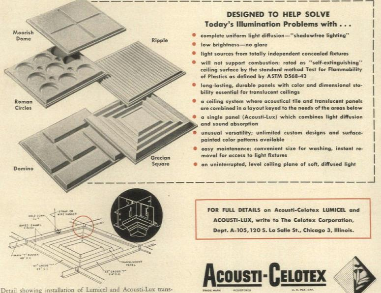
Detail showing installation of Lumicel and Acousti-Lux translucent panels on Alumitee metal suspension system. System consists of rigid 24" x 24" suspended modular, interlocking grid fabricated of extruded aluminum. 1" exposed flanges of "T's" finished in white baked-on enamel. Mechanical hold-down device, easily disengaged for panel removal, keeps translucent panels securely fitted in grid.
