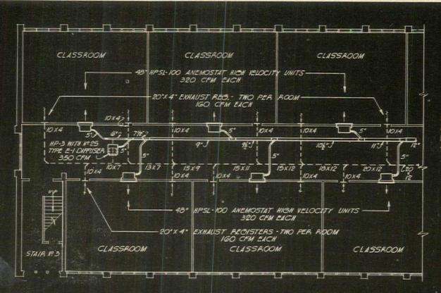
Diagrammatic layout shows corridor distribution of high velocity air for wing of school.
