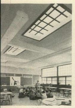
Acting as a daylighting team the Toplite Panels and glass block provide sufficient daylight during normal days without need for artificial lighting.
