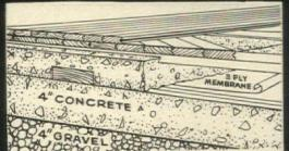
ARCHITECTS AND BUILDERS have discovered that versatile Penta can solve countless construction problems. For instance: when wood screeds are pressure-treated with Penta, they are protected from decay caused by absorption of moisture from on or below grade concrete. Result: Penta-protected screeds provide extra-long life for the gymnasium floor diagrammed above.
