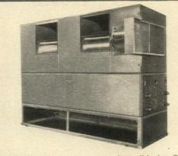
**AIR HANDLING UNITS** for remote air conditioning. Cooling coils available for direct expansion Freon-12, Freon-22, or chilled water. Floor and ceiling mounted units are functionally designed for easy installation and operation. 1,400 to 13,500 CFM.
