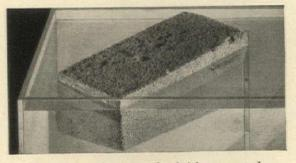
This lighter-than-water fire brick was coated with masonry water repellent made with *Linde* C-25 Silicone, and dried thoroughly. Placed in tank, it repels the water and floats like a cork. Untreated, brick would soak up water and sink instantly.
