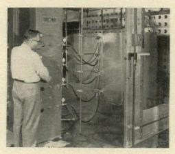
on electrostatically in a prime and color coat, totals no more than .005"—half as thick as regular porcelain enamel and therefore less susceptible to chipping.
