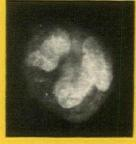
ABOVE: Photomicrograph (microscopic X-ray) of a granule of expanded perlite shows how expansion under 1700°F temperature hermetically seals the air cells (lighter areas), creating ideal insulation. Granule shown was photographed with sodium light.
