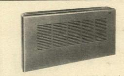
**INDUCTION CIRCULATOR.** Room air conditioning unit operating on high-pressure air induction principle. Used for perimeter cooling and heating of multi-story buildings. Absence of moving parts means long life, quiet operation. 75 to 1000 CFM total air distribution.
