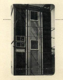
General Bronze testing tower with panel from 2nd National Bank Building ready for air and watertightness test.
