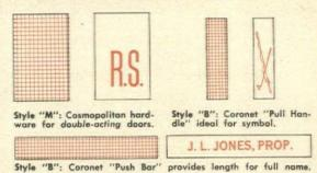
Kawneer offers a choice of four different styles of hardware. The two styles shown have interchangeable face plates. If you wish a face plate to identify any type of business or name, all you do is have artwork prepared. Kawneer will laminate it in plastic, etch it on aluminum, or produce it on any material you desire and in any color. The cross-hatch plate is then merely replaced right on the job with the new design.
