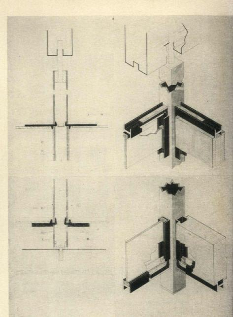
DEMOUNTABLE PARTITION SYSTEM, developed by architects, has only 14 different components, can be moved overnight. It is being patented by owners.
