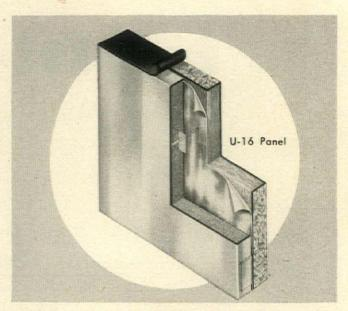
Note how completely the ERIE U-16 Panels meets the major requirements for a curtain wall panel. It is entirely mechanically fastened, reinforced with concrete, insulated, contains an interior reflective barrier and is sealed sufficiently to entrap air as recommended. Separation of the two panel faces reduces throughcontact of metal to a minimum.
