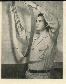
based flooring is as resilient as hardwood and will not crack under extreme temperature changes. The waterproof, nonslip composition is resistant to alkalis and mild acids. It can be used in its natural gray state or dressed up with pigment for applications in hospital rooms, school corridors and auditoriums, and offices. Shipped as two components—liquid rubber and cement powder—Laticrete is mixed on the
