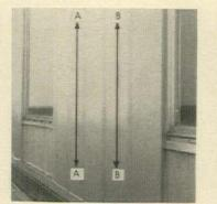
3. TEST PANEL, with slopes under 2%, appears flat. All measurements are in inches.
