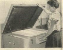
A positive photographic intermediate is produced directly by exposing the "paste-up" in contact with Kodagraph Autopositive Paper, then processing the print in standard photographic solutions. No negative step . . easy room light operation.
