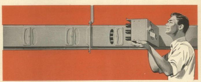
**PLUG-IN POWER WHERE YOU NEED IT**... IN MINUTES! Each section of plug-in duct is 10 feet long with five plug-in openings on each side. Exclusive scarf-lap construction joins sections in a rigid form. Standardized plugs are fastened to casing flanges at plug-in openings. Reinforced fingers engage bus bars for positive pressure contact.
