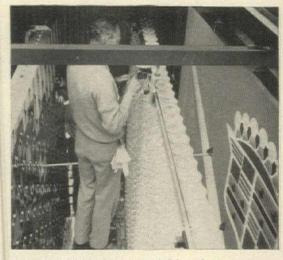
**RUDOLF PABST,** inventor of this unique spectacular, checks a prism rotor. Tough, durable gears and bearings of "'Zytel" nylon resin are used to assure dependable operation of the 49 shafts on which the molded prisms are mounted. Bearings and gears molded of "Zytel" nylon resin require little or no lubrication. Parts molded by American Molding Company, San Francisco, California.
