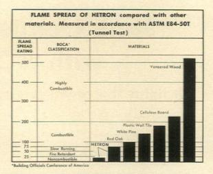
PROPERLY FORMULATED PANELS MADE WITH HETRON can fall within the 20-75 range in flame spread rating (shown by bars representing two typical formulations), as compared with 100 for red oak. For a more complete summary of test results, write us.
