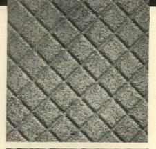
Here is an unretouched photograph of an abrasive tread, purchased on the open market of the type often offered as an equal of Feralun, after the identical acid test. Note the meager amount of abrasive and spotty distribution.
