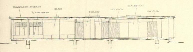
**Slab section** (above) was used instead of two-level scheme worked out for LIFE project (below). Reason: it was decided to use lift-slab method of construction in which flat concrete roof slab is poured on flat floor slab without any need for scaffolding and formwork, then jacked up columns into place. LIFE school used frame roof. In the Bartlesville job concrete slab roof was necessary to match fire rating of existing school to which cluster was attached.
