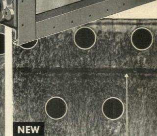
New Delta-Fio Fin. Delta-shaped ridge just ahead of each row of tubes extends turbulence over entire fin surface for uniformheat transfer. Unretouched test photo shows how every inch of fin surface contributes to heat transfer.
