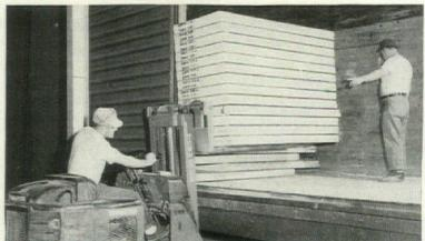
Upper photo shows Tectum after it has rolled through the drying ovens. Complete fabrication requires less than one hour. As a result, as shown in the lower photograph, a railroad car can be loaded with Tectum as it comes off the line—making it available for delivery when needed.
