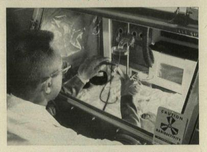
Radioactive work in the Isotope Laboratory Building is done within Kewaunee CBR enclosures
