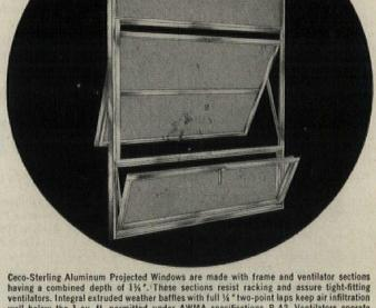
Ceco-Sterling Aluminum Projected Windows are made with frame and ventilator sections having a combined depth of 1½ ". These sections resist racking and assure tight-fitting ventilators. Integral extruded weather baffles with full ½ "two-point laps keep air infiltration well below the 1 cu. ft. permitted under AWMA specifications P-A2. Ventilators operate easily, because of counter-balancing design. All glass is in the same plane.
