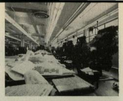
In-line layout moves copy in straight path from composing to press. All mechanical departments are on plant's first floor.
