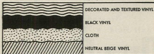
Cross section of "Tontine" drapery material
