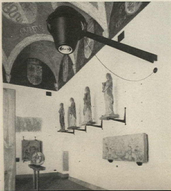
Dual fixture , one of the few that are very evident, illuminates indirectly above, spots below.
