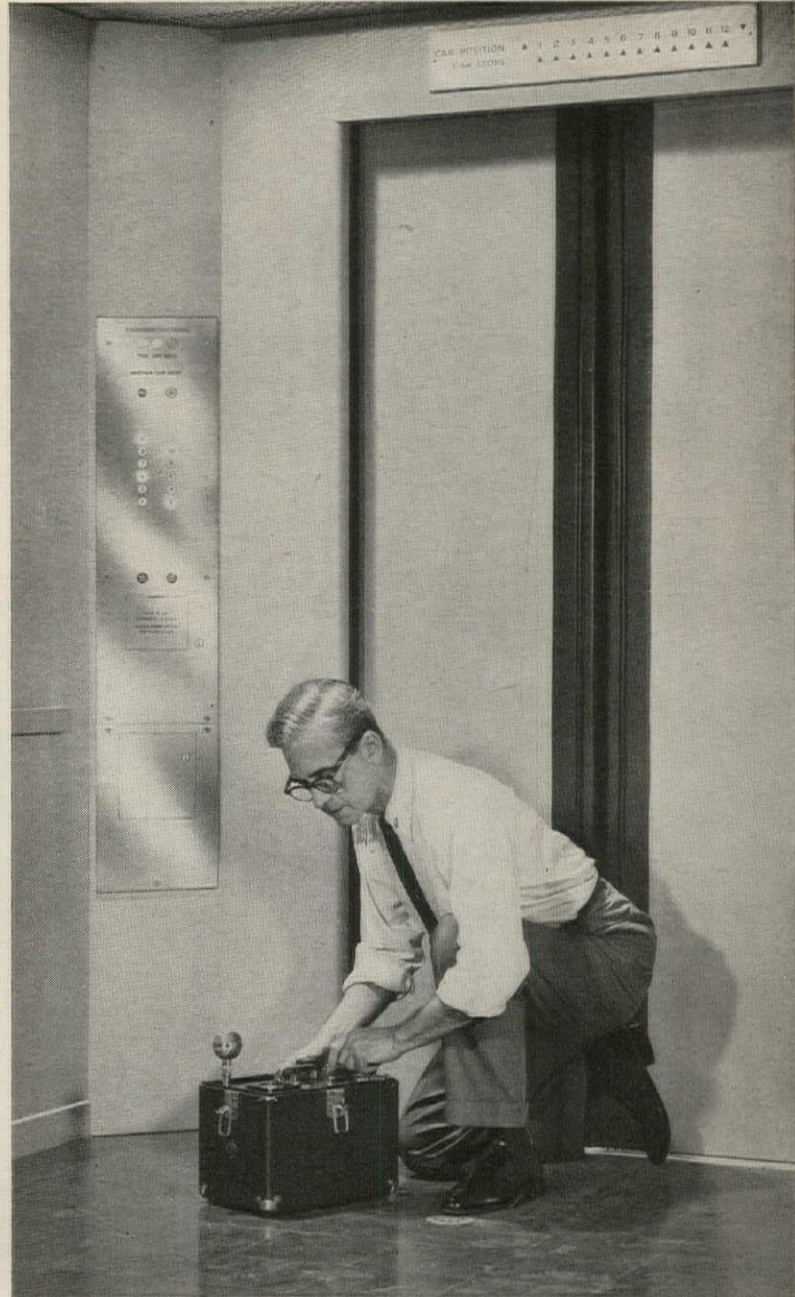
Sound level meter readings were also taken while elevators were traveling from floor to floor in normal operation.
