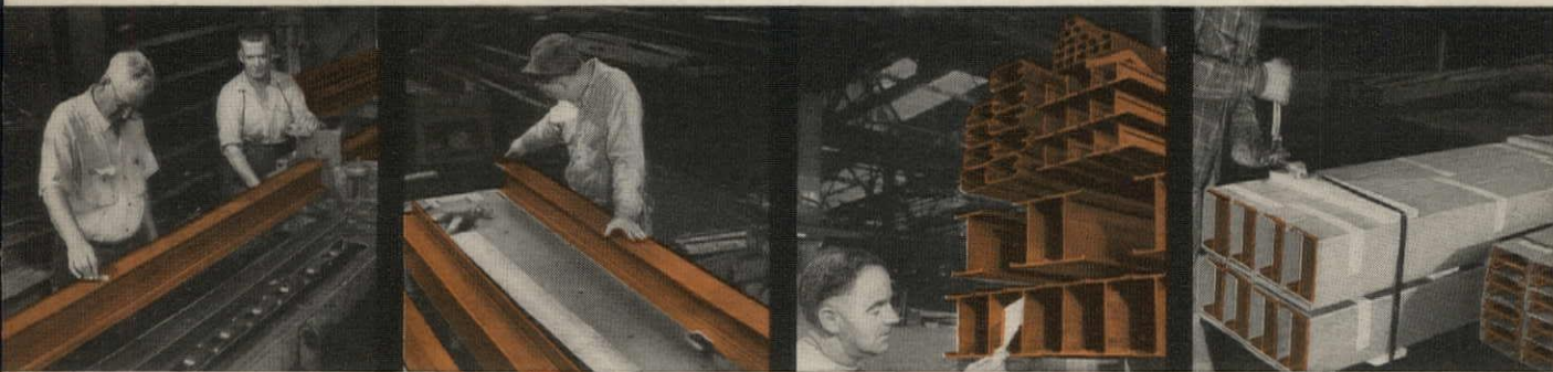
STRAIGHTENING PROCESS involves drawing shape through a second die.
