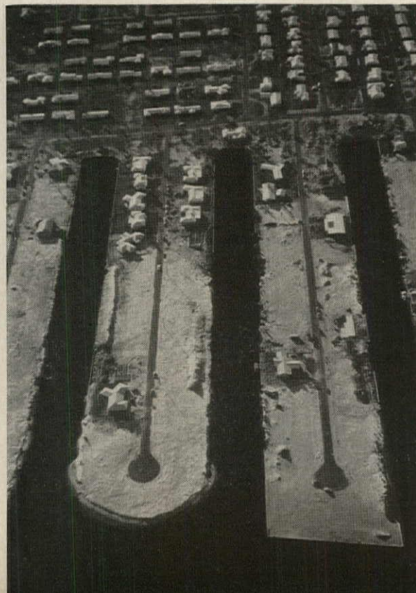
Bulldozer and dredge carved these luxury housing peninsulas out of mangrove swamp at Ft. Lauderdale, Fla.
