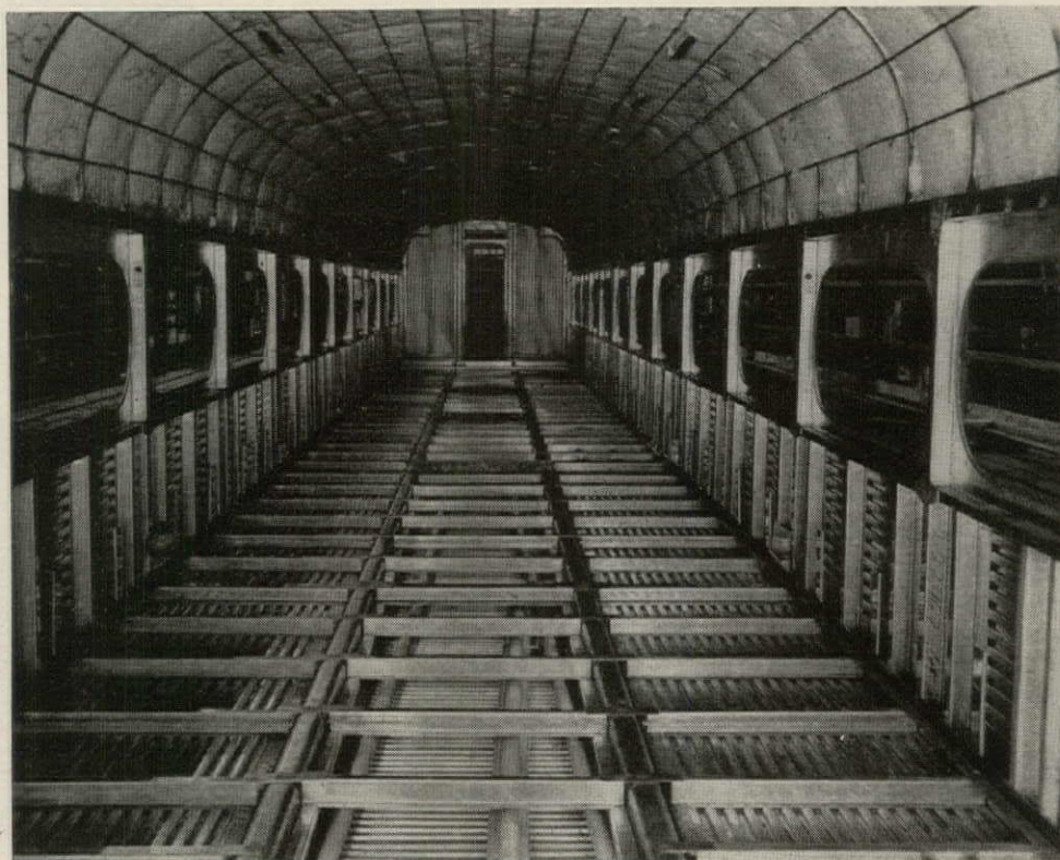
Interior structure is of high-strength stainless steel. Underframe is efficient, two-sill span which extends uninterrupted from one end of car to the other.
