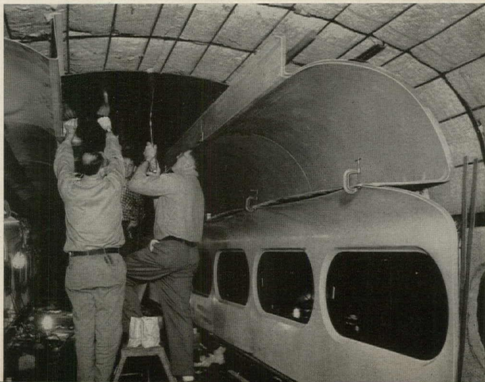
Two plastic panels cover most of each window bay. First extends from floor, includes underside of rack; second covers rack, plus ceiling and half of air duct.
