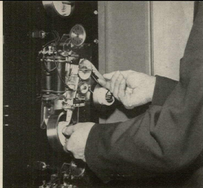
Commuter runs can be pre-programmed. Trains are tape-controlled from remote station.
