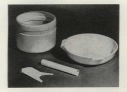
TECHNIQUES used in conventional glass making—drawing, pressing and casting—are all applicable to the new crystalline materials.
