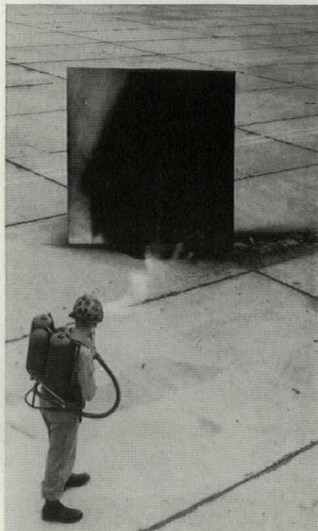
After Marine's flame-thrower blast . . . the panel stands—smudged but in good shape.
