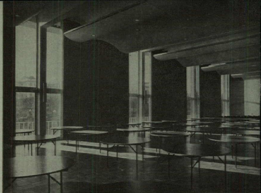
Acoustical ceiling in the multi-use auditorium accommodates troffer lighting for general use and stage lighting for theater-in-the-round.
