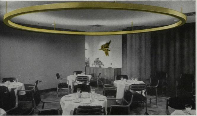
novel and decorative arrangement of indirect lighting, utilizing a channel-shaped ring of bronze, provides uniform light on the tables this dining room designed by Architect J. Gordon Carr, N. Y. The reflected light has a softening influence on all colors of materials, luding the bronze. The antique bronze flying geese on far wall are modern welded sculpture by Barbara Lekberg, N. Y.
