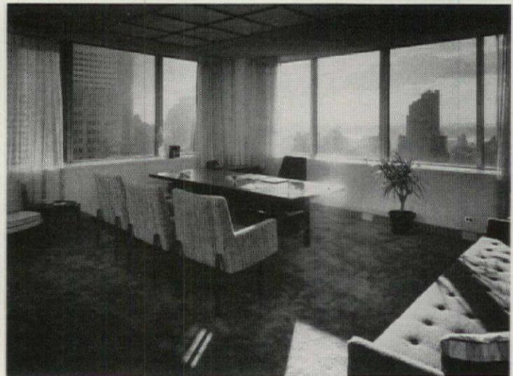
**Glass ceilings:** Secretarial space in Corning's second-floor general offices is set off from exterior cubicles by glass framed in movable metal partitions. Acoustical ceilings of glass fiber incorporate rectangular panels of Corning's new light-diffusing lens materials. Glass fiber is used also in insulation, wall coverings, and furniture.
