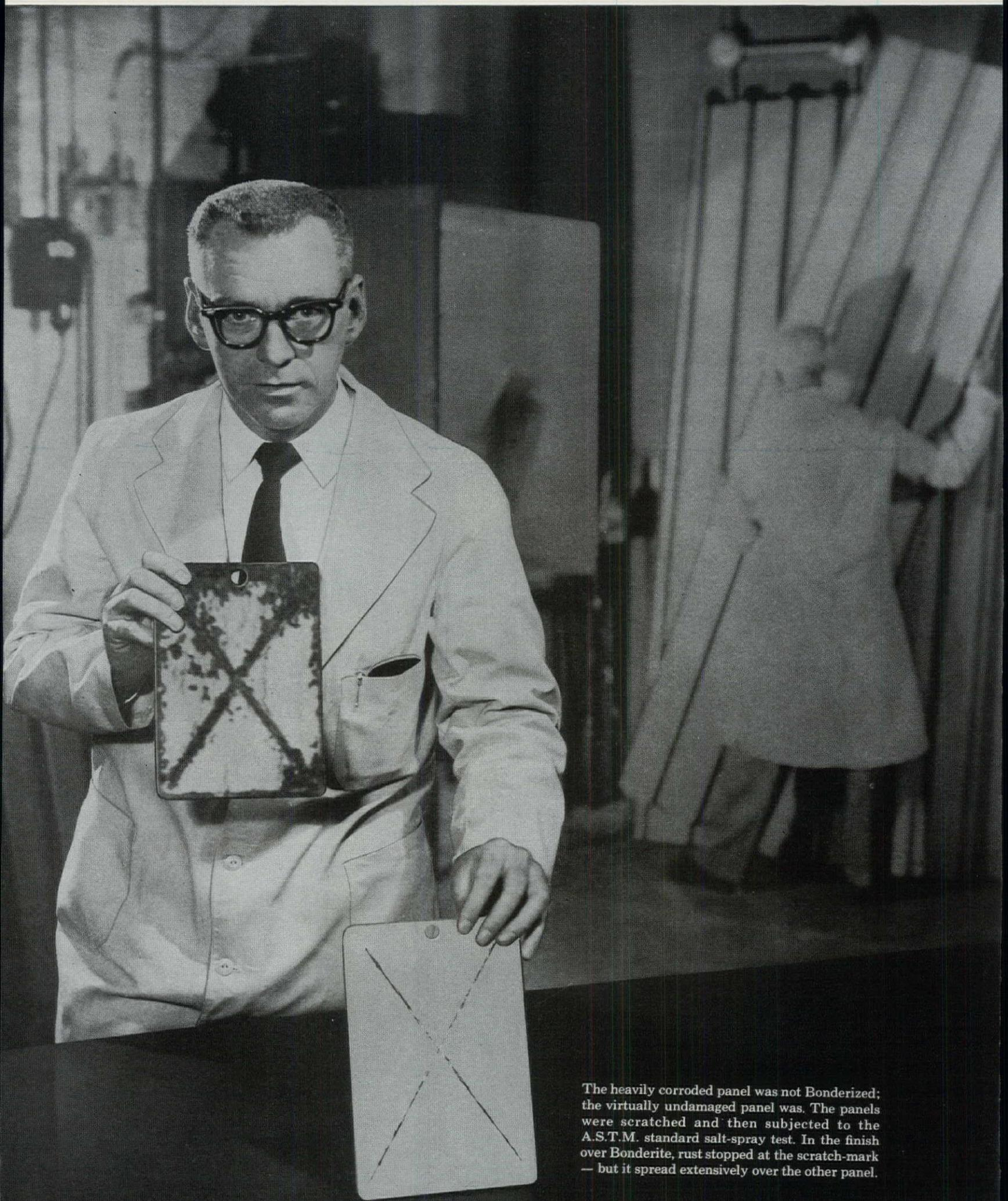
The heavily corroded panel was not Bonderized; the virtually undamaged panel was. The panels were scratched and then subjected to the A.S.T.M. standard salt-spray test. In the finish over Bonderite, rust stopped at the scratch-mark — but it spread extensively over the other panel.
