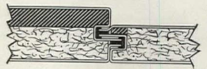
Method of joining vinyl gaskets.
