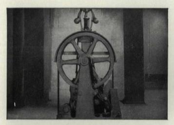
MEET THE GOVERNOR... Here's the "boss" of the "safety" shown at the lower left. It's constantly alert to car speed and its normal function is to stop the car at the next floor landing in the event of overspeed. However, should overspeed be excessive, its trigger-like reflexes will activate the "safety" immediately and automatically.
