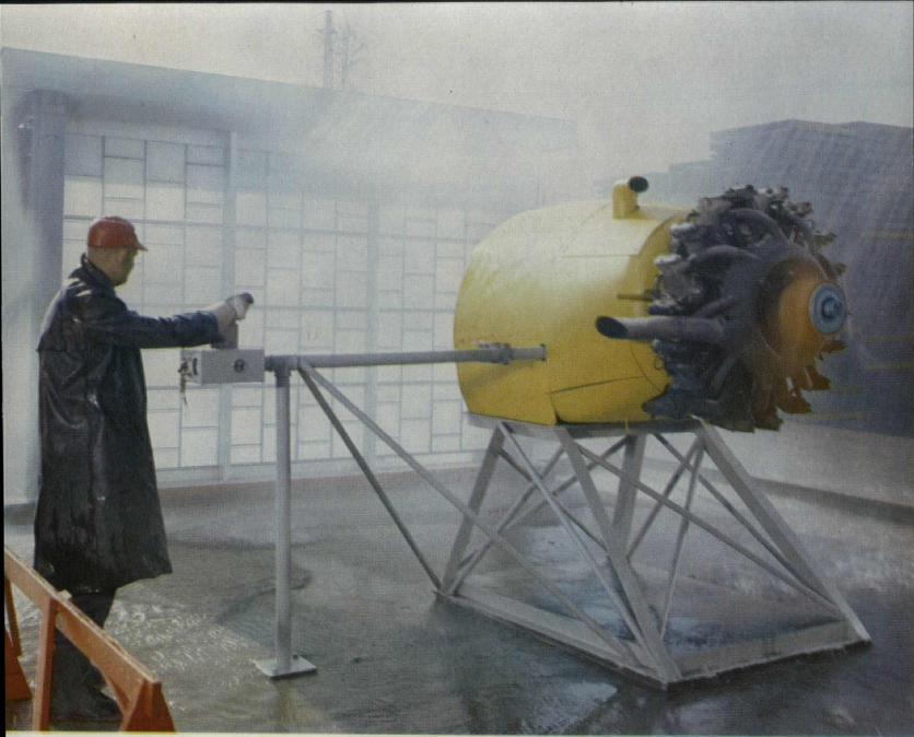
Aircraft engine hurls gallons of water against THINLITE wall at near-hurricane velocity in weather-resistance test.
