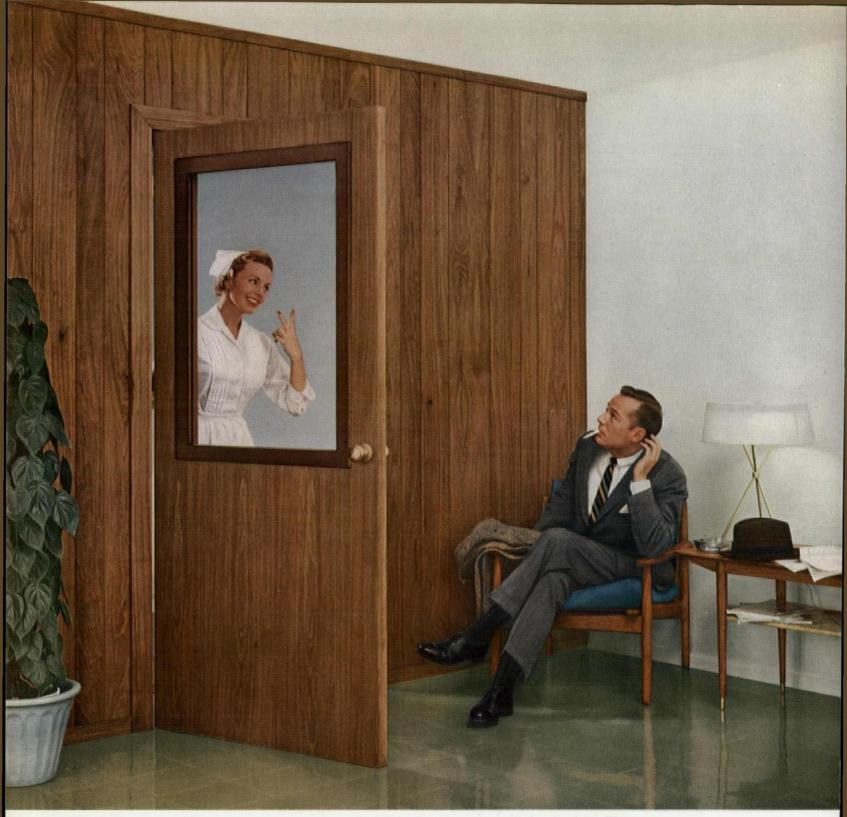
VISION PANELS in Weldwood Fire Doors come in five sizes (up to 30" x 36") for Class "C" openings, and in two sizes (up to 100 sq. inches) for Class "B" openings. Paneling shown is new Algoma-made fire-resistant Weldwood prefinished walnut V-Plank®.
