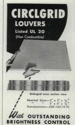
Circlgrids are thermo-formed from 2 sheets of vinyl and fused electronically to a center vinyl membrane for structural strength and rigidity—yet weigh only 3 ½ oz./sq. ft. Many leading lighting equipment manufacturers are licensed to sell and distribute Circlgrid.
