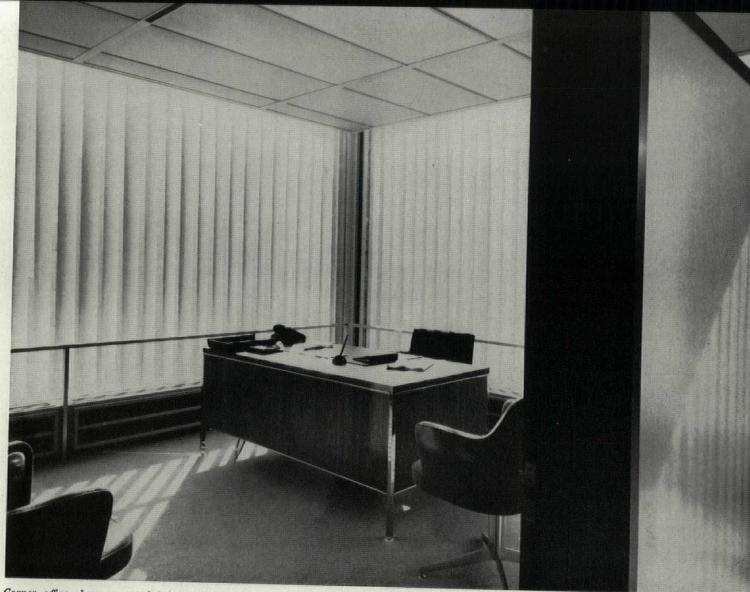
Corner office shows a careful integration of low heating-cooling units, guard rails, blinds, furniture, and ceiling return-air slots.
