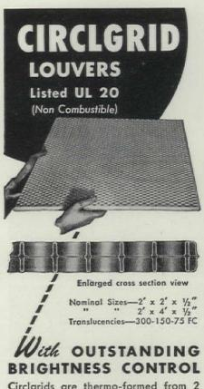
Circlgrids are thermo-formed from 2 sheets of vinyl and fused electronically to a center vinyl membrane for structural strength and rigidity—yet weigh only  $3 \frac{1}{2}$  oz./sq. ft. Many leading lighting equipment manufacturers are licensed to sell and distribute Circlgrid.
