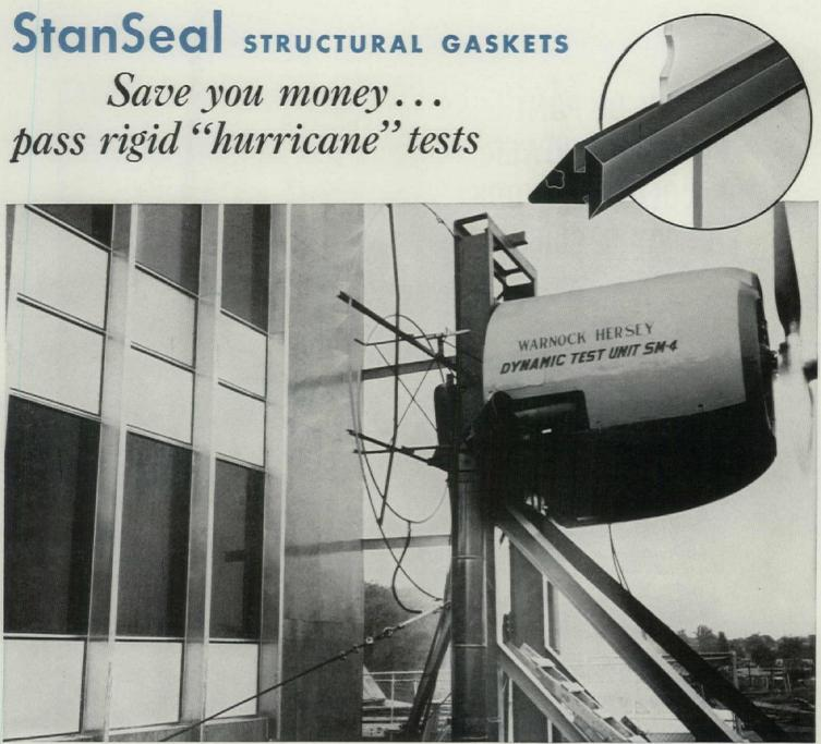
You can save up to 30 cents a square foot on curtainwall construction through the use of STANSEAL structural neoprene gaskets. The job will go up faster, easier-and you need have no fear of troublesome, expensive leaks.
