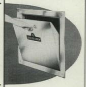
Electrical interlocking prevents the use of more than one intake door at the same time in multi-story buildings. Wilkinson electrically interlocked chute doors automatically lock when any one door is opened. When this door closes and after a predetermined time delay, all doors are unlocked.
