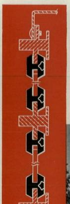
Sash, spandrel and glass "closed" with standard INLOCK 760161
