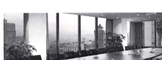
The board room is a bright and cheerful place to work because of the wide expanse of window area. SOLEX heat-absorbing glass used here absorbs about 50% of direct solar radiation and reduces glare.
