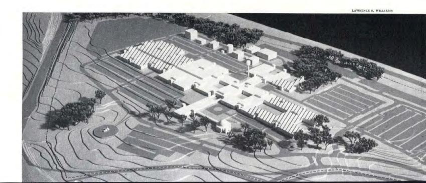
"Research is a messy business. The building should not be allowed to get in the way." He extends this principle both to the laboratory partitions, made of 2<sup>3</sup>/<sub>4</sub>-inch-thick gypsum board, to which shelving can be easily attached and which are relatively lightweight and movable, and to the ceiling system, which consists of movable ventilating, lighting, and acoustical units.
