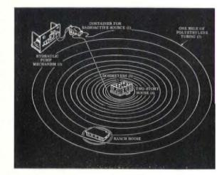
Checking fallout protection: scientists at Technical Operations, Inc. simulate and evaluate radioactive fallout with a source of radioactive cobalt in the plastic hose. The cobalt is pumped round and round through the system, and detectors within the structure (below) measure degree of radioactivity at various points. This is part of fallout research program of OCDM.
