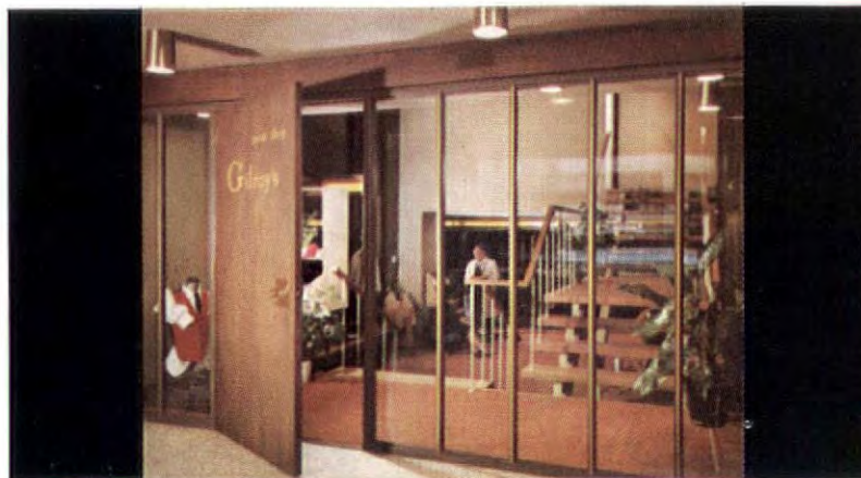
NUWELD® MESH polished, wired glass by A-SG puts a sleek facade on Gilroy's Men's Shop in Seattle's new LOGAN BUILDING. Nuweld Mesh was specified for its fine optical quality, fire retarding properties, and the clean, modern lines of its wired pattern. Architects: Bittman & Sanders.
