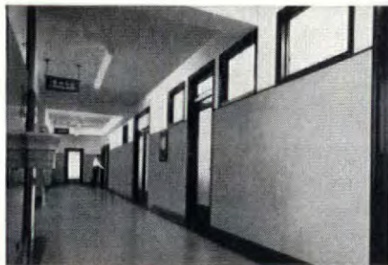
Each corridor has two sets of controlled lights — one ON every day — one near windows, ON when it's dark outside.
