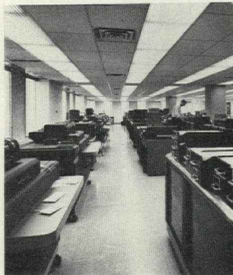
Machine heat is drawn off through false floor.
