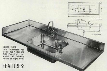
Invisible joints, no dirt-catching lap joints or solder seams, raised and rolled pre-formed edges, 4-inch backsplash, choice of right or left endsplash. sloping decks, heat resistant underseal, choice of Haws faucet fixtures, vandal proof fixture locking, chrome plated trim, famous Haws quality!
