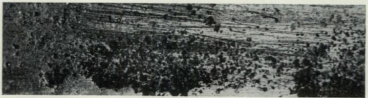
ANOTHER SPECIMEN OF THE SAME CONCRETE was treated with a coat of typical sealer. After 500 strokes, the surface showed wear of 0.0007 inch, the equivalent of 2/3 of 1 mil. The surface appeared unbroken. But, look what happened when the sealer was stripped away. Photo is of block abraded after stripping by paint and varnish remover. The concrete showed erosion to a depth of 0.0027 inch; or the equivalent of 2.7 mils. The surface was broken and badly worn away.
