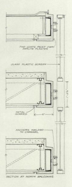
Worm's-eye-view construction photo (right) shows how paired beams transmit load of cantilevered balcony decks to column between them. Structural details are shown in plan (left) and in section (above). Discontinuity of balconies is emphasized (opposite page) by white horizontal band of middle deck, revealed between upper and lower sun screens.
