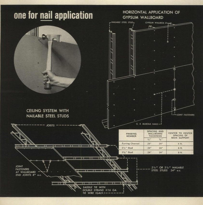
Cutouts are provided in these studs to allow passage of conduits and utility piping. With either system, wallboard goes on fast and easy to complete the job in less time.
