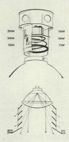
Plastoveil trim is a perforated lath around the aperture, to which plaster, acoustical tile, or other ceiling materials may be keyed. The fixture plate remains accessible but the whole fixture is less obtrusive.
