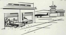
Airport Emergency. Combining electronically operated doors with emergency alarm signals saves valuable seconds for many airport fire stations. A signal from the airport tower simultaneously opens doors, turns on lights and triggers alarm bells in fire station often located at other end of airfield.
